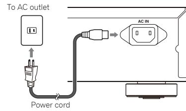
**1 Plug the supplied power cord into the AC IN socket on the back of the unit.**
